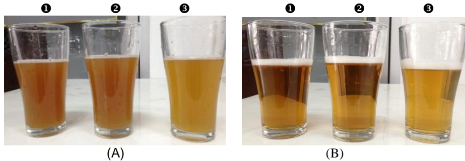
Figure 5 Comparison of color and turbidity between before (A) and after (B) filtration of beer (①=Rice beer from wort mashing at 65°C, ②= 75°C, ③=Beer from standard congress wort)
