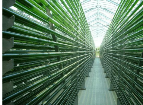
Figure 7 Tubular photobioreactor (From:www.brae.calpoly.edu/CEAE/images/biofuels3.gif)
