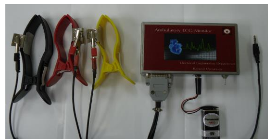
Figure 4 Sensor clips and the instrumentation amplifier with filter in a shielding case.
