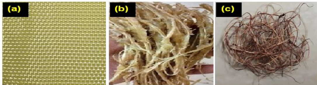
Figure 1 (a) Virgin Kevlar fiber, (b) Before extracted Cucurbitaceae fiber, (c) Extracted Cucurbitaceae fiber
