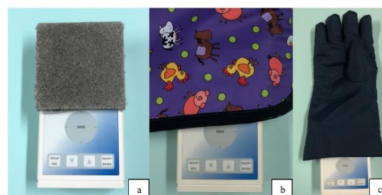
Figure 2 Set up for radiation quantity measurement of the Bismuth composites (a) lead apron (b) and lead glove (c)
