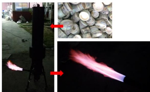
Figure 10 Flame caused by producer gas combustion
